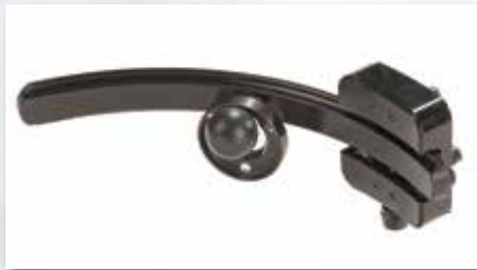
The rail rotates with the headrest. The base remains stationary. The knob underneath permits locking at any position of rotation.
